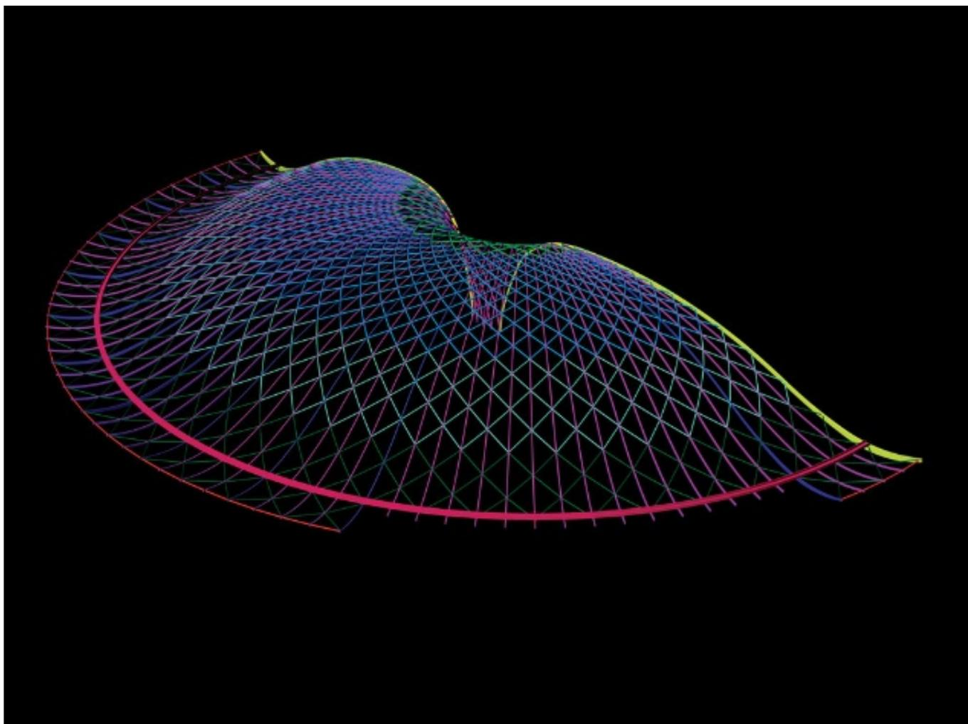
Bentley technology was used to design the new roof of King's Cross station by John McAslan.
