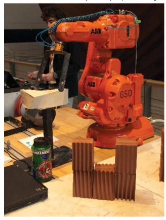
Ceramics 2.0's industrial robot uses taut wire to cut clay.
